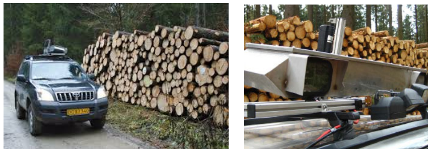
Fig. 3. Camera log measurement system by the company Dralle [15]
