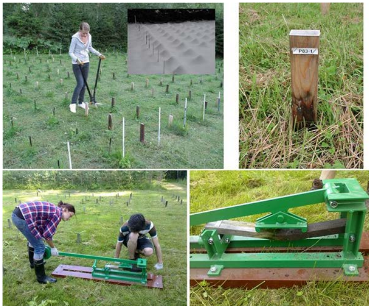
Fig. 2. Overall view of EN 252 decay field test at Punkaharju in summer and winter time, grass maintenance, Scots pine stake in close view and strength measuring with bending apparatus
