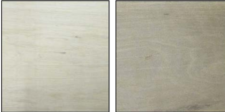
Fig. 4. Colour change as a result of acetylation on hornbeam wood (left: untreated; right: acetylated)
