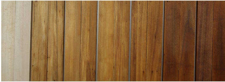
Fig. 2. Colour change of poplar wood due to different heat treatment schedules in linseed oil
