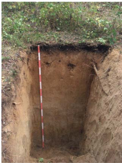
Fig.3. A typical soil profile of sandy texture in the southern part of Amur region.
